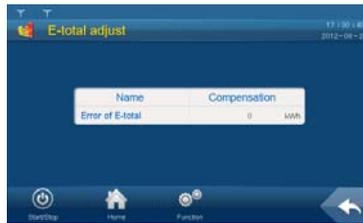
Tap the cell below the "Compensation" and the keypad appears. Enter the energy compensation by tapping the keypad;
