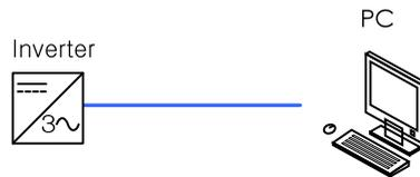
**Fig. 3-5** Ethernet communication of one inverter
