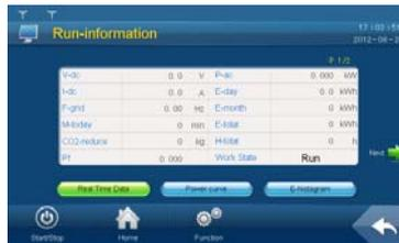
**Step 3** Tap "Power curve" and enter into the power curve sub-menu;
