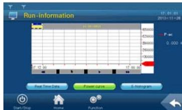
**Step 4** Tap "E-histogram" and enter into the electricity histogram sub-menu.
