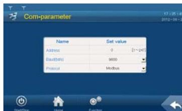
Three parameters pertinent to RS485 serial port communication can be set according to the parameter range shown on the display.
