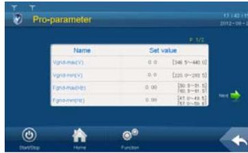
Set the protection parameter by tapping the pop-up keypad and tap ENTER to confirm setting. Tap “Prev” or “Next” to turn pages up or down.
