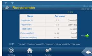
**Step 4** Set the running parameter by tapping the pop-up keypad and tap ENTER to confirm setting. Tap "Prev" or "Next" to turn pages up or down.
