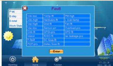
The fault window will appear with the present fault in red.
