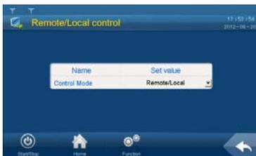
**Step 5** Select the control method through the pull-down list.
