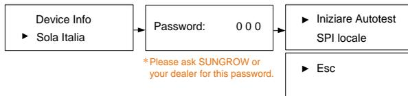
**Touch ENT** to start the auto test. If the inverter is in the status of “Error” or “Turn off”, it cannot start the test and a prompt interface will appear.
