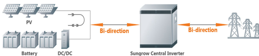
Fig-6: DC ESS interface and PCS mode of SG6800HV-MV
